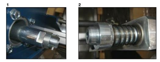
1 Drive spindle  $\rightarrow$  pivot center for Heidelberger (for other presses pivot center is different) 2 Tail spindle  $\rightarrow$  pivot center for Heidelberger (for other presses pivot center is different))
