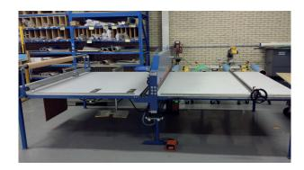
**Gluing of bars:** The glue is applied using a glue gun and a set of glue nozzles. This ensures that the proper glue stripe (width and thickness) required by every individual bar is applied onto the blanket prior to mounting and pressing the bar.
